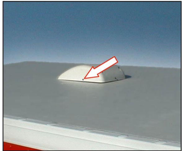
Illustration VE-35 Roof Vent (Exterior View)
