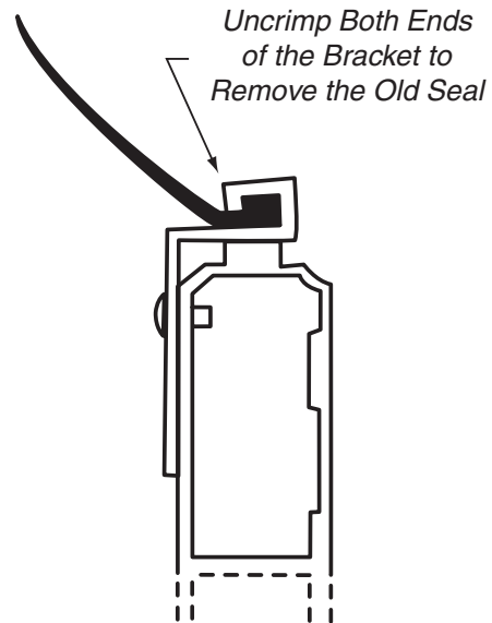
Illustration DR-95 Top Seal on Roll-up Door
