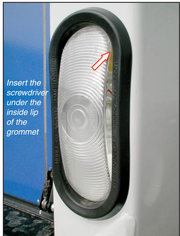
Illustration LI-25 Back-up Light (Grommet Mount)
