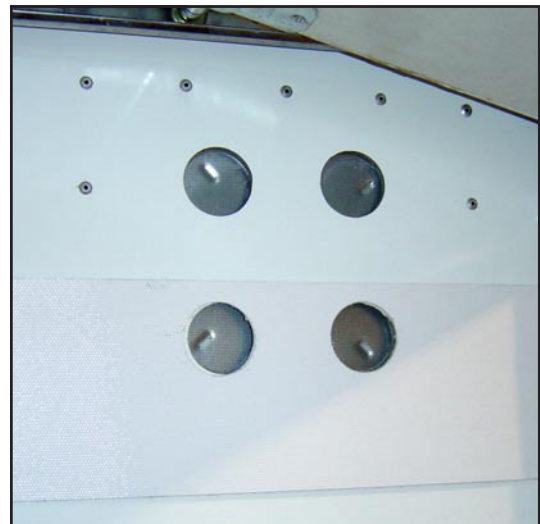
Illustration VE-10 Lowered Butterfly Side Vent Interior View
